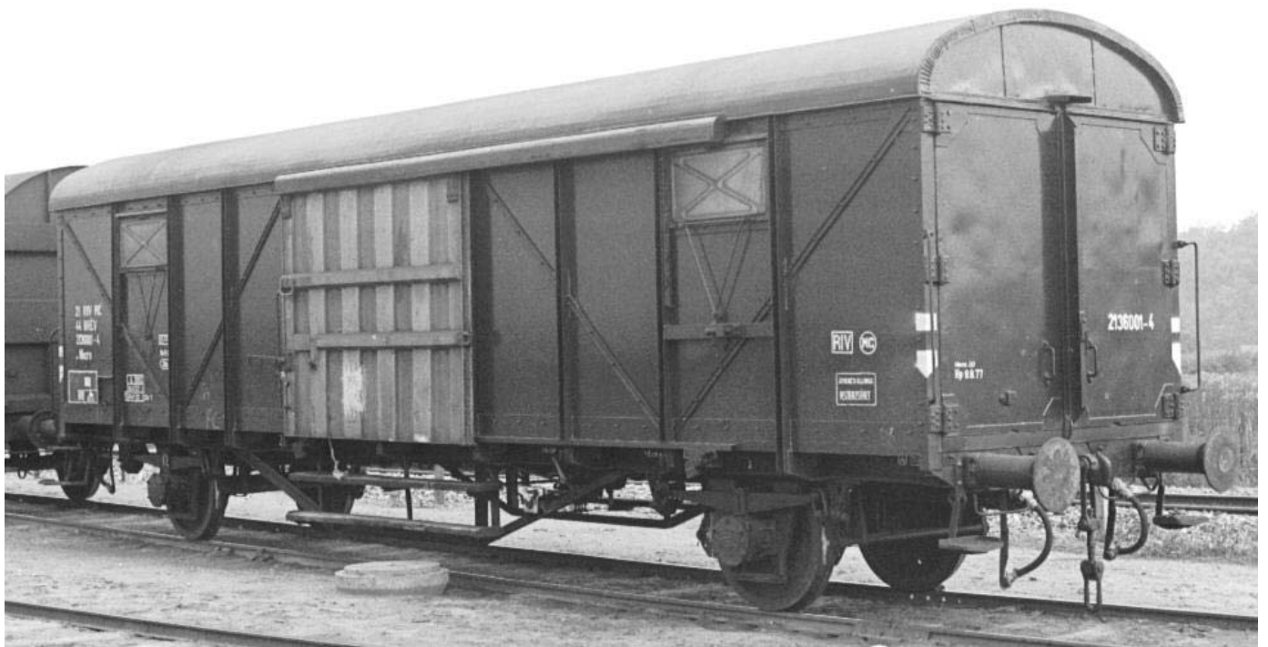
21 44 BHÉV 2136001-4 •Hbcrs , with tare 15220 kg and load limit 22,0 t. DK-Sakskøbing 07.10.1974 © Per Topp Nielsen
