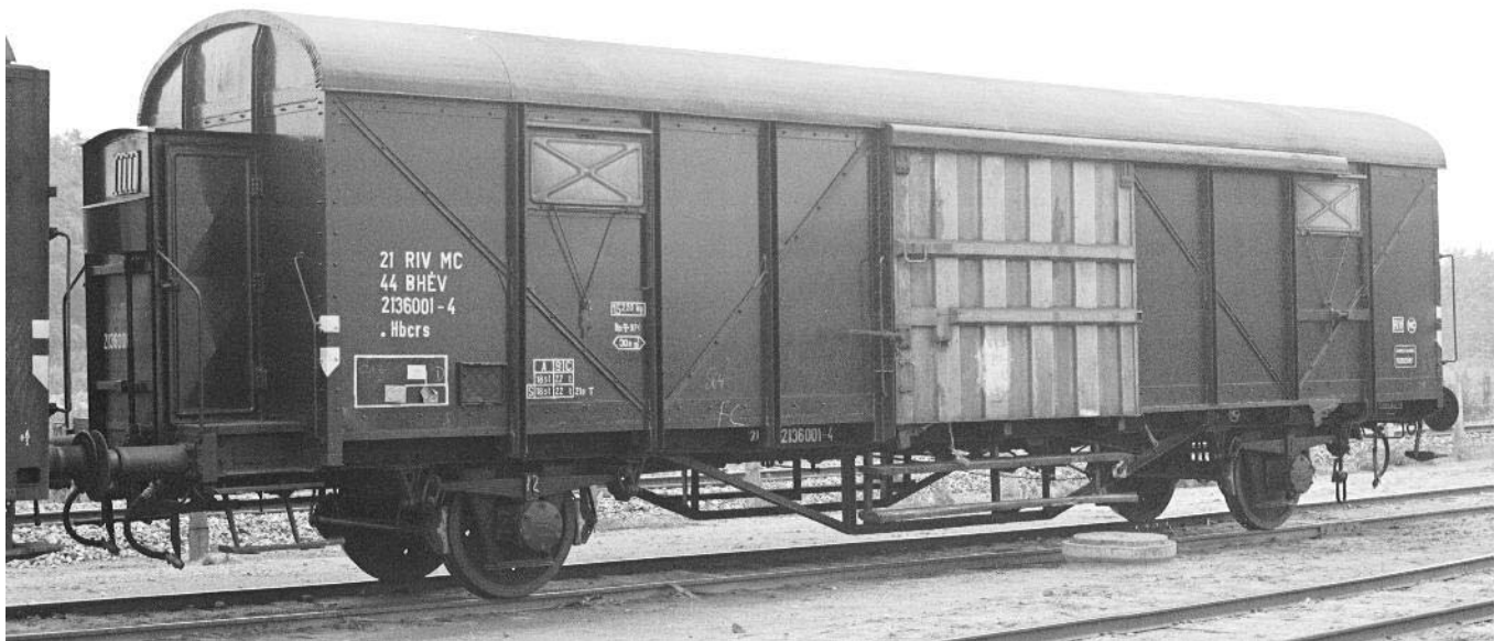
21 44 BHÉV 2136001-4 •Hbcrs , with tare 15220 kg and load limit 22,0 t. DK-Sakskøbing 07.10.1974 © Per Topp Nielsen
