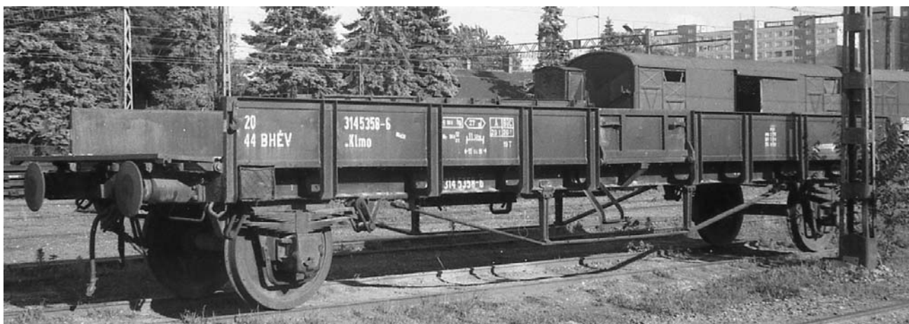
20 44 BHÉV 3145358-6 •Klmo , with double stacked leaf springs. Filatorigát 24.06.1990 © Per Topp Nielsen
