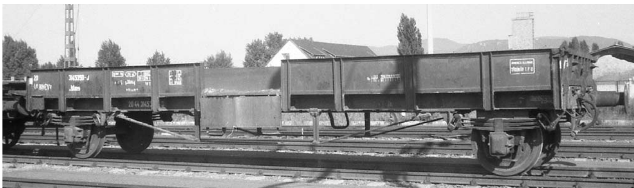
20 44 BHÉV 3145350-3 •Klmo , with triple stacked leaf springs. Szentendre 25.06.1990 © Per Topp Nielsen
