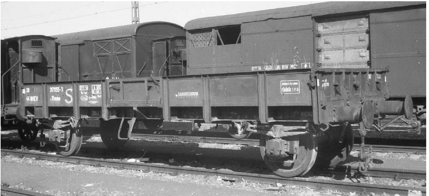
20 44 BHÉV 3171155-3 •Klmmo, with double stacked springs and 60 cm buffers. Szentendre 25.06.1990 © Per Topp Nielsen
