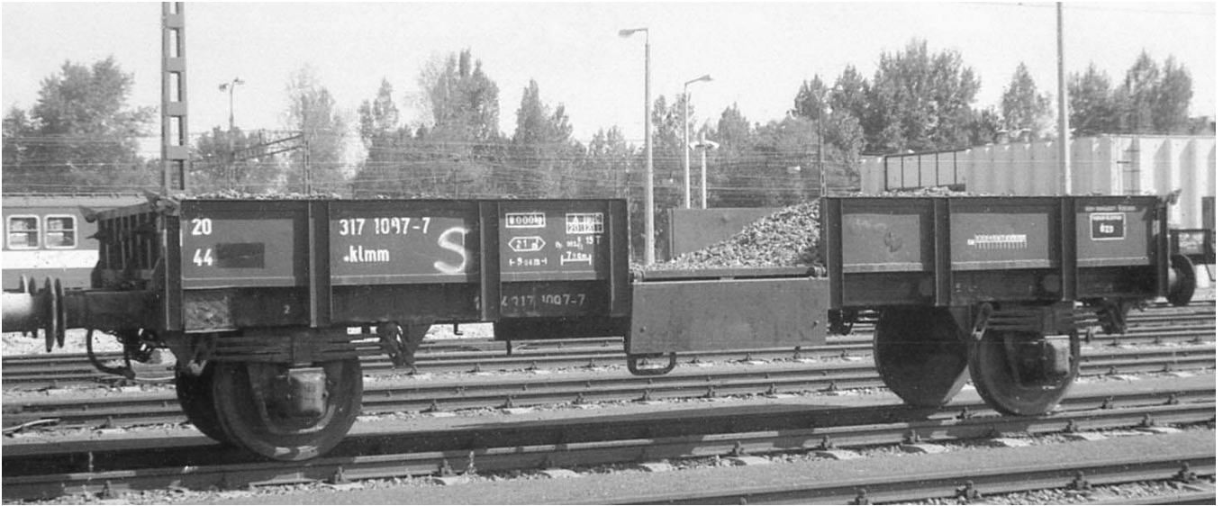
20 44 BHÉV 3171097-7 •klmm, with triple stacked leaf springs and short buffers. Szentendre 26.07.1989 © Per Topp Nielsen
